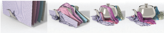
Fig. 19. For 2D manifolds, the integration domain degenerates, effectively reducing the required quadrature points compared to volumetric models. Here, five high-resolution tablecloths (totaling 150K DOFs) interact with a teapot. Our method captures intricate folding patterns in real-time, requiring only 57 ms per time step.
