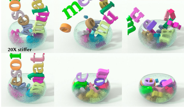
Fig. 14. Our three-level quadrature scheme robustly captures both high-frequency and low-frequency propagation of \varphi at each node. Therefore, our method is not sensitive to the stiffness of the model. In this example, we drop letters of “Awesome simulation” into a glass bowl. Letters in the top row are 20 \times stiffer than those in the bottom row. There are 534K DOFs in this test, and our method robustly simulates both scenes using 22 ms (top), and 19 ms (bottom).
