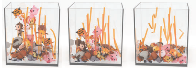
Fig. 11. “Animal crossing”. The subspace reuse technique allows our solver to handle stiff materials and deformable bodies with ease. This example includes 33 animal toys, 10 elastic ribbons, 678K DOFs, and one million elements. Both our method and PD-IPC [Lan et al. 2022b] produce penetration-free animations, while our method is 12× faster than PD-IPC on RTX 3090.
