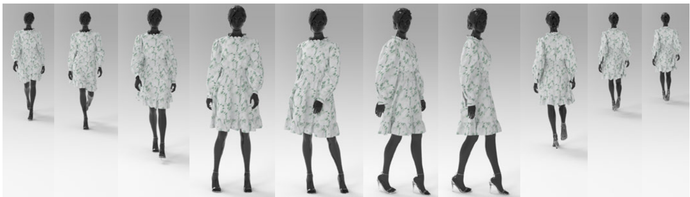
Fig. 1. Fashion show. We present a new GPU-based cloth simulation framework with projective dynamics. Our method is able to simulate high-resolution cloth meshes at an interactive rate. With a non-distance-based barrier formulation, we can replace a large portion of traditional CCDs with the partial CCD procedure, which is much less expensive. The subspace reuse strategy relaxes the low-frequency errors effectively at the cost of single-digit milliseconds. Our method also features a residual forwarding trick to alleviate the damping issues generated by early termination and small-step line search filtering. In the teaser, we show an animated scene of the virtual fashion show. The model, dressed in a soft and light midi skirt, walks to the front and then turns around. These series of movements cause complex fabric dynamics, vividly showcasing the design concept of the garment. The garment is of high resolution and has 340K vertices. The corresponding simulation involves over one million unknowns, and detailed local wrinkles can be well perceived. With a time step of \Delta t = 1/200 sec, the simulation runs at 4.8 FPS. Please refer to the supplementary video for the corresponding animations.
